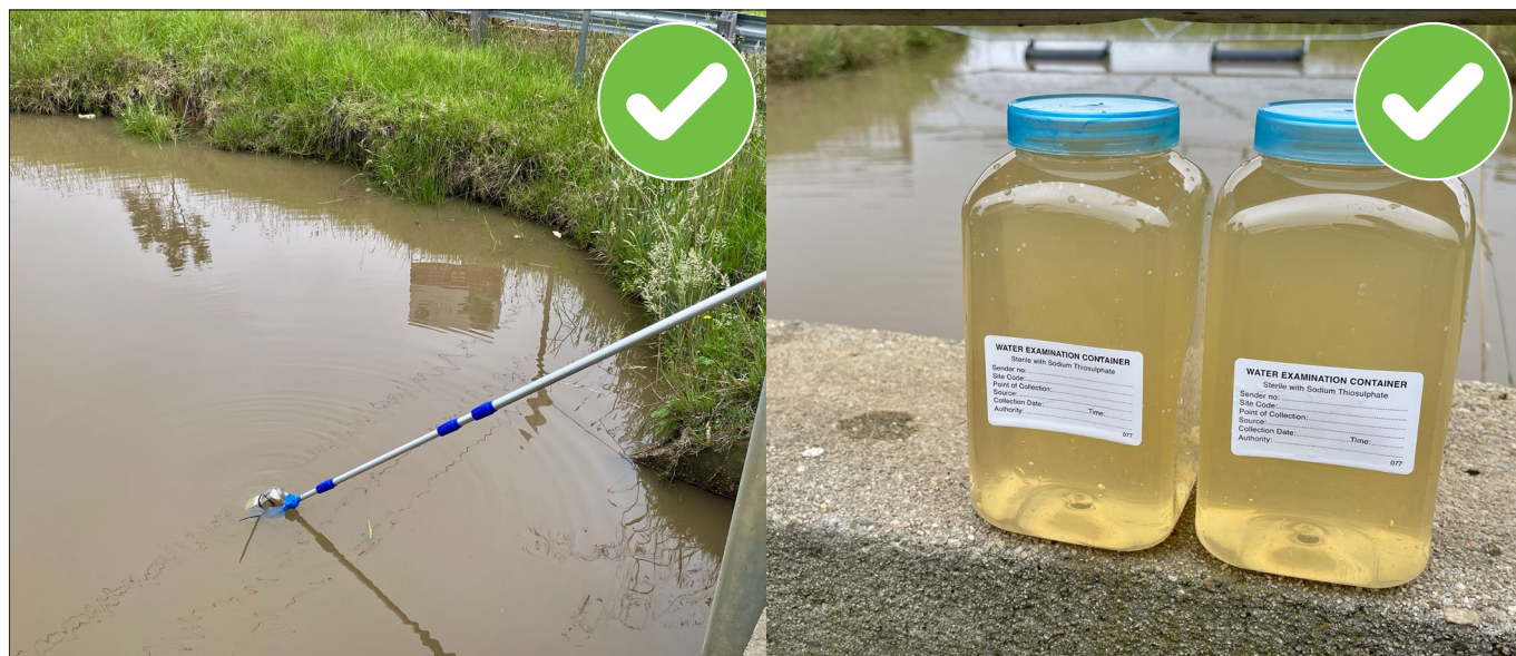
Image C18.1 | Using a telescopic pole allows for safe and controlled collection of water from the centre of the pond, minimising disturbance to sediment and reducing the risk of contamination from the pond perimeter.
