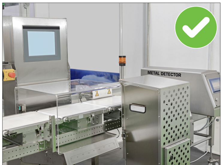
Image C3.1 | In-line metal detectors are used in fresh produce operations to identify and remove physical contaminants.
