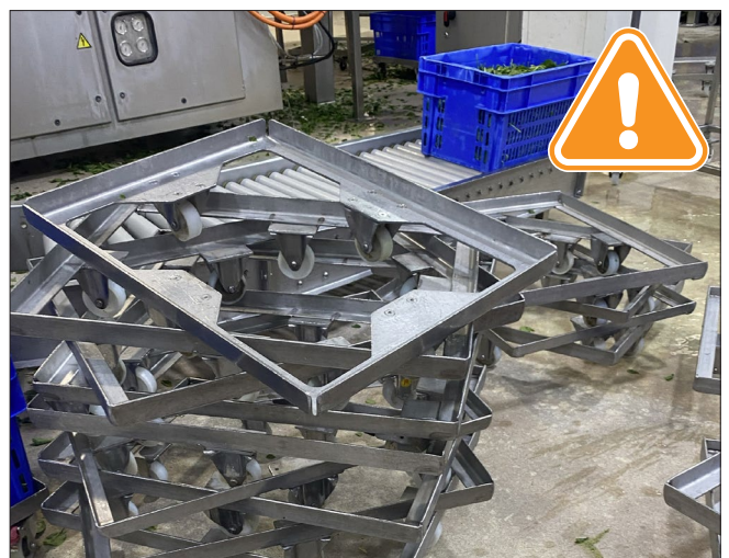
Image C9:4 | Unacceptable practice example with untidy or inadequately maintained internal areas that may harbour pathogens and attract pests.
