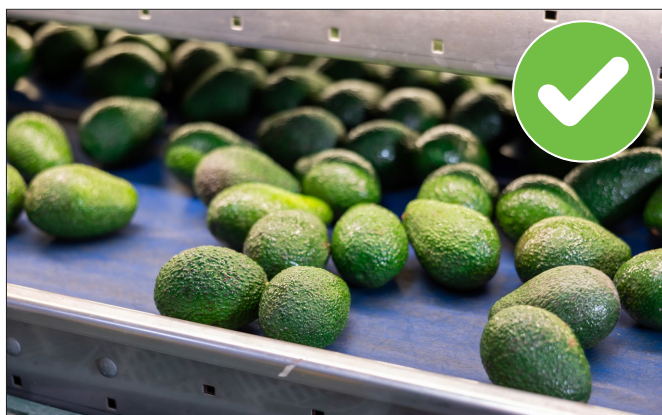
Image C10:1 | Good practice example of a packing line constructed from smooth rubber; a non-absorbent, durable material.
