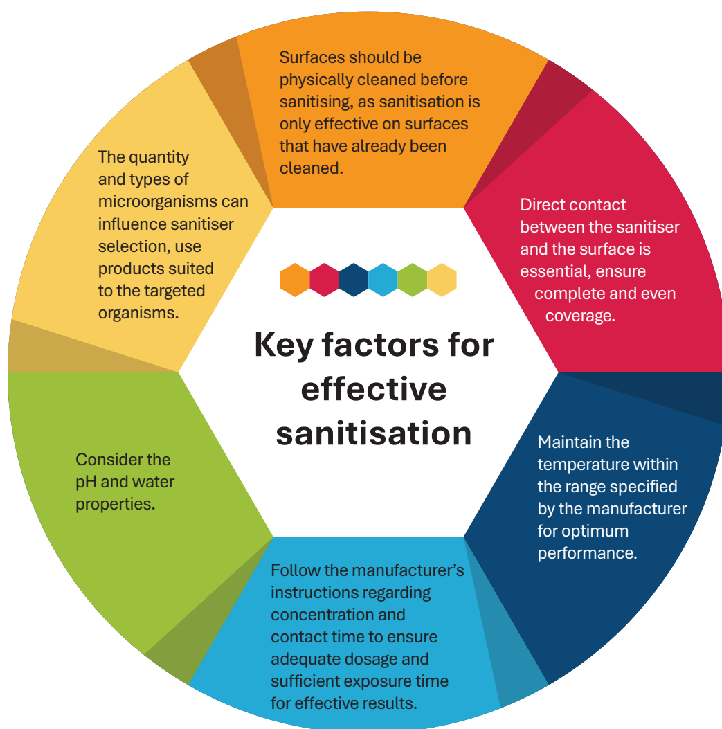
Figure C10.1 | Key factors for effective sanitisation.
