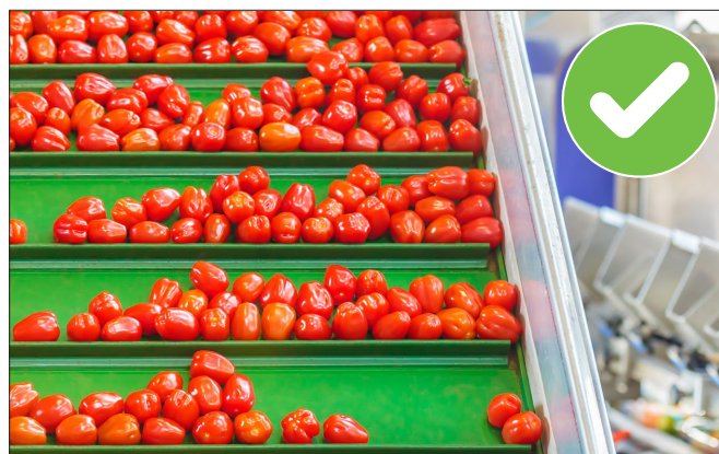
Image C10:2 | Good practice example of a packing line constructed from stainless steel. This surface is easy to clean and maintain, reducing the risk of contamination.
