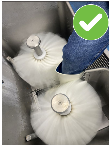
Image C14:8 | Cleaning and sanitising footwear before entering production areas reduces the risk of pathogen contamination.
